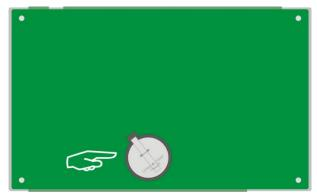
Figure 136 Remove the battery
