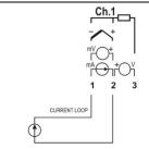
The connection for the channels is made in the terminals in accordance with the figure at the left. Please observe the correct polarity of the connection.
