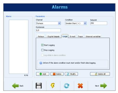
Figure 63 Alarms Configuration - Log control settings
