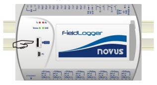
Figure 129 Insert the USB flash drive
