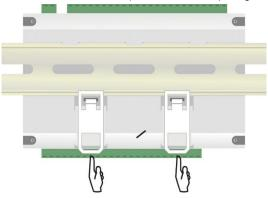
Figure 3 DIN rail installation
