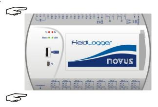
Figure 134 Remove the connectors
