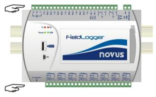
Figure 127 Remove the connectors (1)
