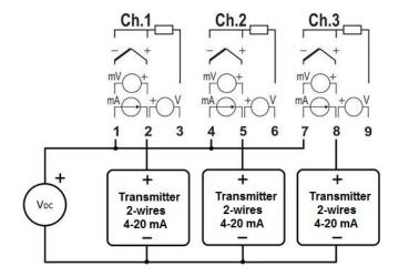
Figure 21 Auxiliary power supply powering 4-20 mA (2-wire) transmitters
