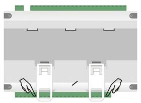
Figure 1 DIN rail installation
