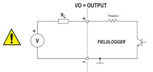
$\textbf{Figure 18} \qquad \text{Connection of a load $R_L$ to a digital output}$
