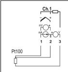
The connection for the channels is made to the terminals in accordance with the figure at the left. The 3-wire connection from the Pt100 sensing element to the **FieldLogger** input guarantees the cancellation of the error caused by the resistance of the wires. All three wires must have the same gauge and length.
