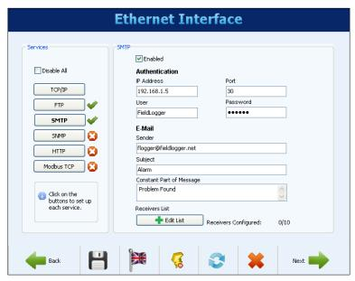
Figure 44 Ethernet Interface - SMTP Configuration
