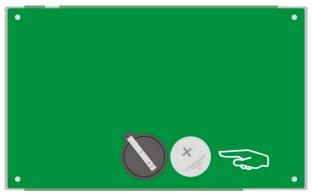
Figure 137 Replace the battery
