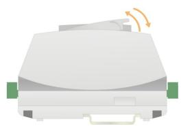
Figure 11 Attaching and detaching FieldLogger HMI (side view)
