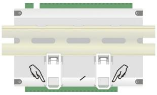
Figure 133 Detach FieldLogger from DIN rail
