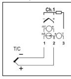
The connection for the channels is made in the terminals in accordance with the figure at the left. Please observe the correct connection polarity.
