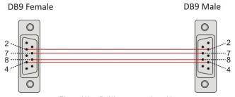
Figure 112 Building an extension cable
