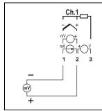
The connection for the channels is made in the terminals in accordance with the figure at the left. Please observe the correct polarity of the connection.
