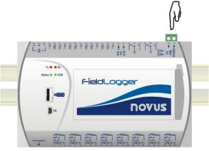
Figure 130 Reconnect the connector and the power supply cable
